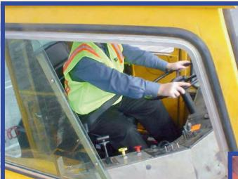
So why wear a seatbelt ? It's just common sense. A seatbelt is proven protection against injury. Use your head...use your seatbelt !!! Whether you're driving a forklift, UTR, yard truck or any other piece of equipment in the yard. If it has a seatbelt ...
