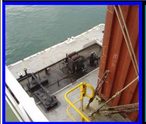
Lashers: Control all bars. Don't let them drop or bounce. Steel bars deflecting off steel decks can skip a long way. They can end up on a bunker barge or in the middle of the highline!
