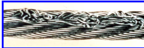
Flattened, crushed wire or damaged sling eyes
