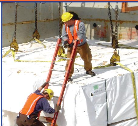
*Before using a ladder in the hold make sure it is secured.
