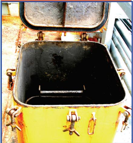
*When entering the hold through a hatch, the ladder lid needs to be secured.
